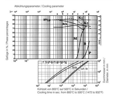
A....Austenite B....Bainite K....Carbide P....Perlite M....Martensite RA....Retained Austenite
