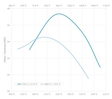
Holding time 3 x 2 hours Specimen size: square 25 mm
