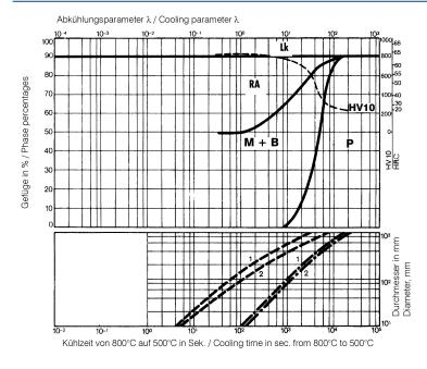
Lk... Ledeburite carbide RA... Residual austenite A... Austenite B... Bainite
