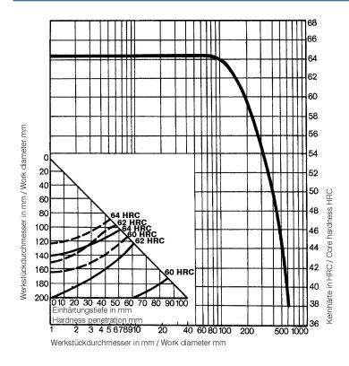
Hardening temperature: 1030°C / 1886°F Quenchant: ——— Oil ----- Air
