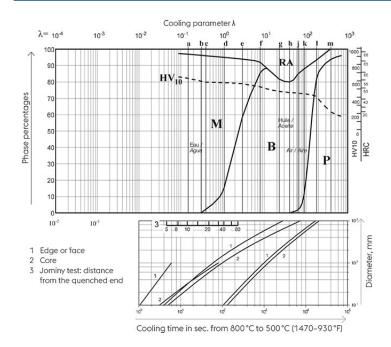
A... Austenite B... Bainite K... Carbide M... Martensite P... Perlite
