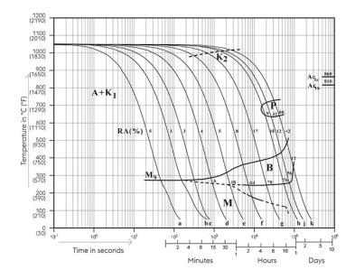
Austenitising temperature: 1050°C (1922°F) Holding time: 30 minutes 5...100 phase percentages 0.5...400 cooling parameter, i.e. duration of cooling from 800 - 500°C (1472-932°F) in s x  $10^{-2}$
