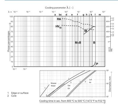
A... Austenite B... Bainite K... Carbide M... Martensite P... Perlite RA... Retained austenite
