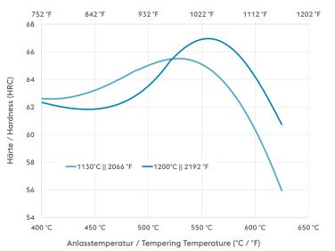
Holding time 3 x 2 hours Specimen size: square 25 mm
