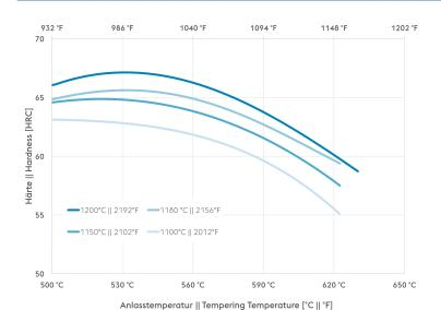
Holding time 3 x 2 hours Specimen size: square 25 mm
